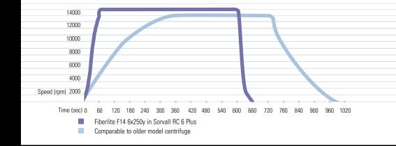
Fast acceleration and deceleration rates in the Sorvall RC 6 Plus centrifuge ensure that samples experience optimal RCFs within the shortest period of time, increasing your throughput.
