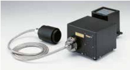
Transmitted light detection unit External transmitted light photomultiplier detector and 100 W halogen conventional illumination, integrated for both laser scanning and conventional transmitted light Nomarski DIC observation. Motorised exchange between transmitted light illumination and laser detection. Simultaneous multichannel confocal fluorescence image and transmitted DIC acquisition enabled.
