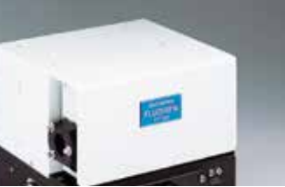
SIM Scanner Second dedicated scanner for photostimulation, synchronised to the FV1200 main scanner for simultaneous photostimulation and confocal image acquisition. Independent fibre-optic laser introduction port. Dichromatic mirror within motorised optical port of the scan unit required for introduction of laser into main scanner.
